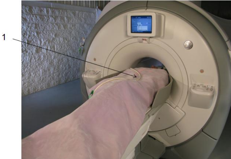
Figure 2-53: 1 = ECG cable with no loops
