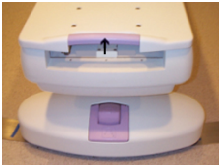
Figure 2-36: Cradle release handle, 0.7T OpenSpeed tables
