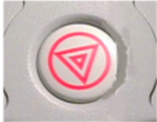
Figure 2-30: Emergency Stop button
