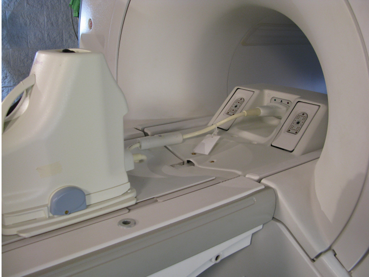
Figure 2-49: Coil cable with no loop
